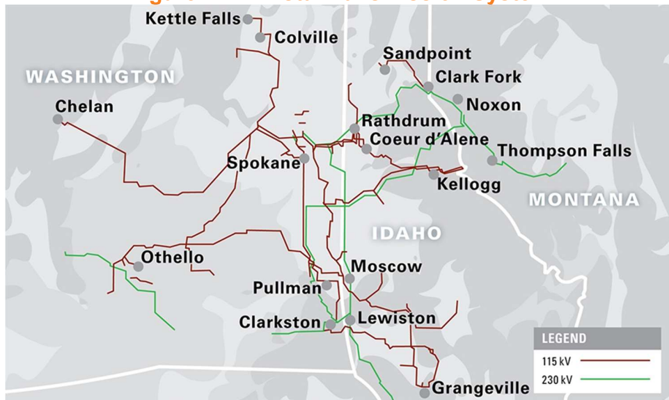
Figure 7.1: Avista Transmission System
