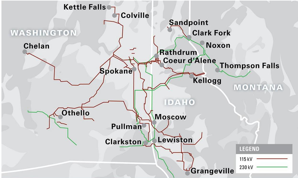
Avista owns an 11 percent interest in 495 miles of double circuit 500 kV lines between Colstrip and Townsend, Montana. The transmission system includes switching stations and high-voltage substations with transformers, monitoring and metering devices, and other system operation-related equipment. The system transfers power from Avista's generation resources to its retail load centers. Avista has network interconnections with the following utilities:
