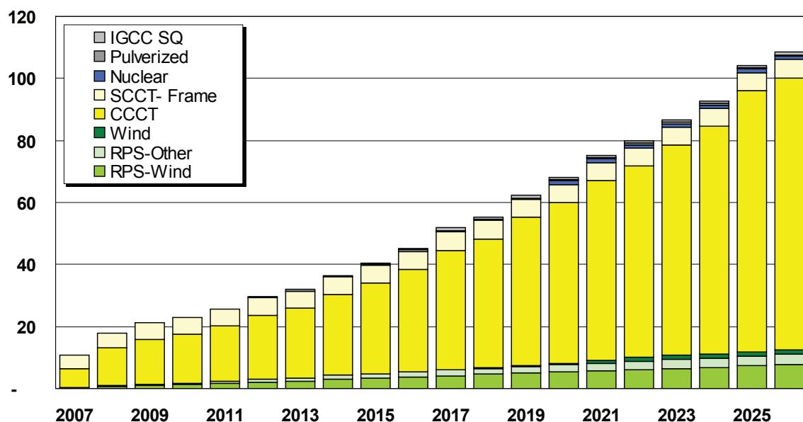
Figure 6.30: Western Interconnect Generator CO<sub>2</sub> Emissions Forecast
