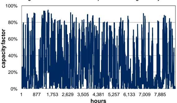
Figure 7.12: 2012 Actual Wind Output BPA Balancing Authority<sup>5</sup>
