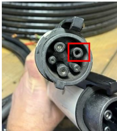
Figure 18: Connector pin damaged (missing internal piece) after utilization of a non-Tesla adapter.
