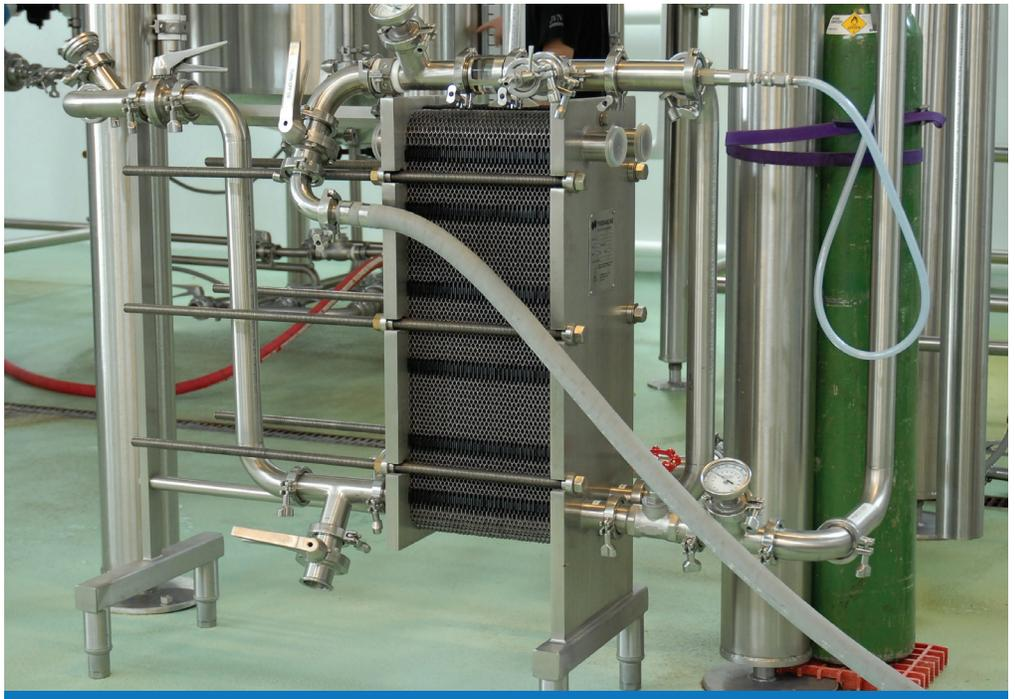
The heat exchanger gives a master brewer more precise control when cooling down wort.
