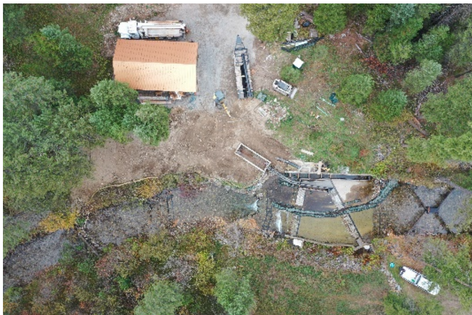
Aerial view of Graves Creek permanent weir trap and associated fish handling facility.
