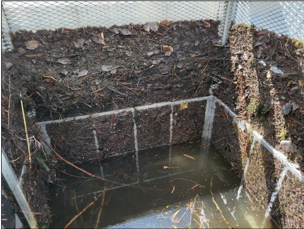
Figure 1. Inside of the trap box after 24-h of fishing during a time of moderate instream debris loads.
