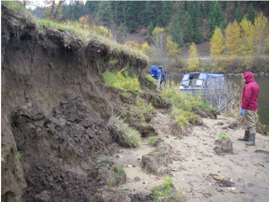
Photographs taken from IDEQ's St. Joe Riverbank Erosion Potential Inventory (IDEQ 2011) showing extreme erosion potential, based upon the BEHI bank score, at the Bank Pin No. 9 Site.
