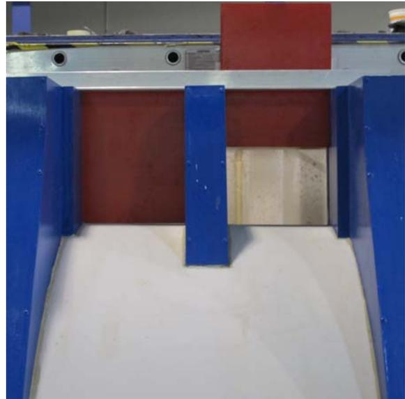
**Photo 6:** Individual slide gates used to control spillway discharges.
