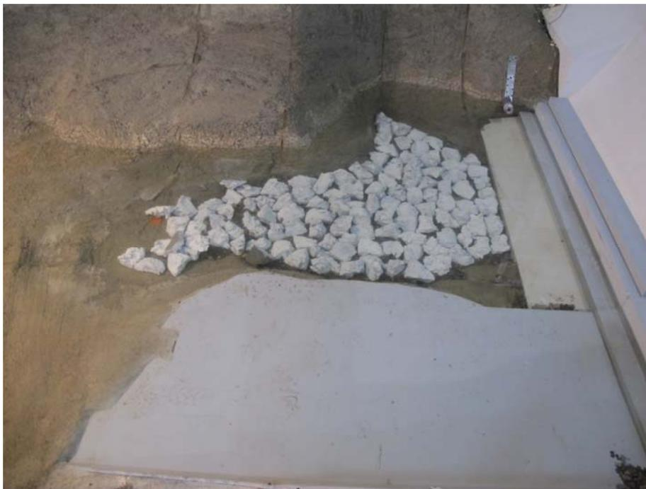
**Photo 2:** Mobile bed following 5.5 hours (prototype) of 50,000 cfs spillway discharge.
