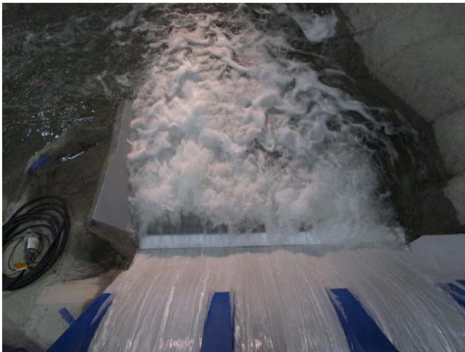
**Photo 2:** 25,000 cfs Spillway Discharge – Bays 3-8 – ramped surface jet flow and surface jump.
