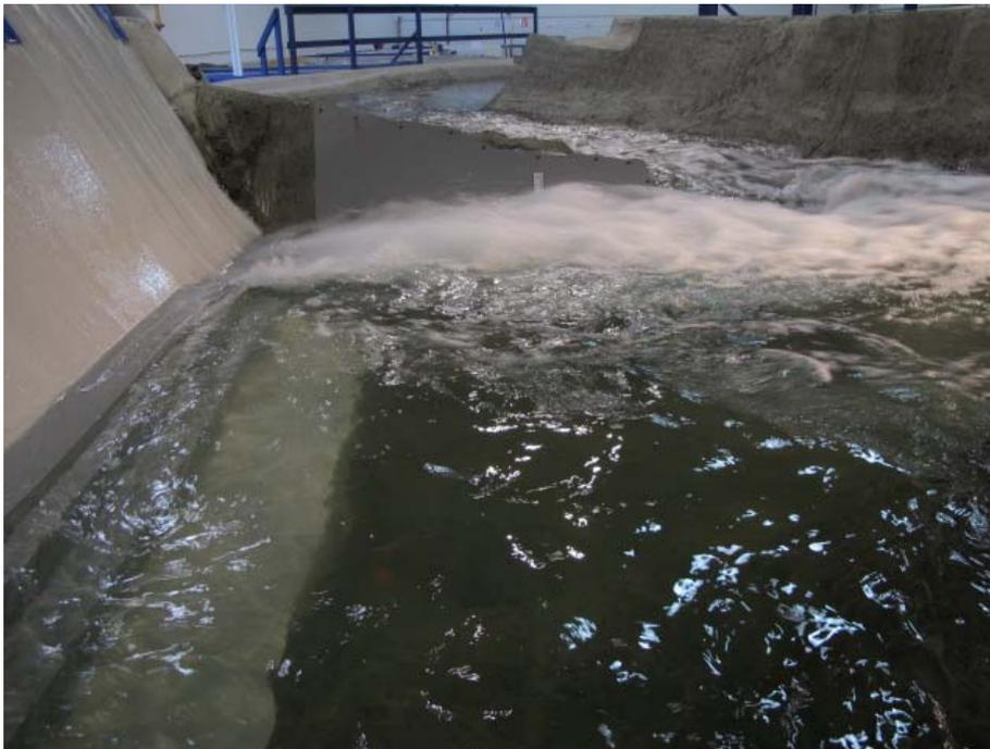
**Photo 4:** 10,000 cfs Spillway Discharge – Bays 7-8 – skimming to ramped surface jet.
