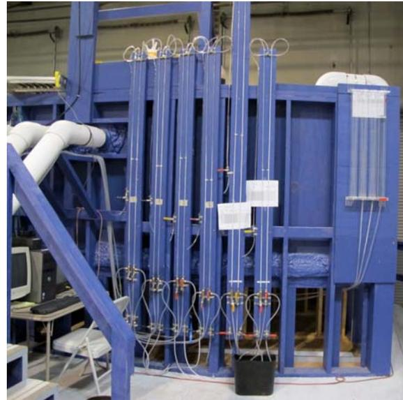
**Photo 2:** Manometer boards used to measure deflection and measure flow.
