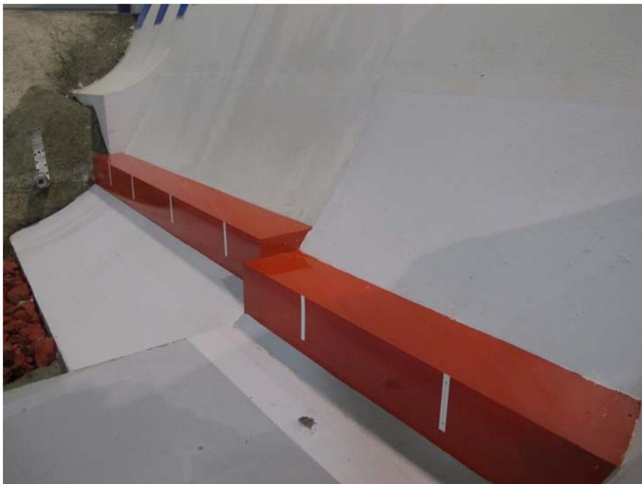
**Photo 2:** The final configuration consisted of an elevation 1368 ft deflector on Bays 7 & 8 and an elevation 1373 ft deflector on Bays 3 through 6.
