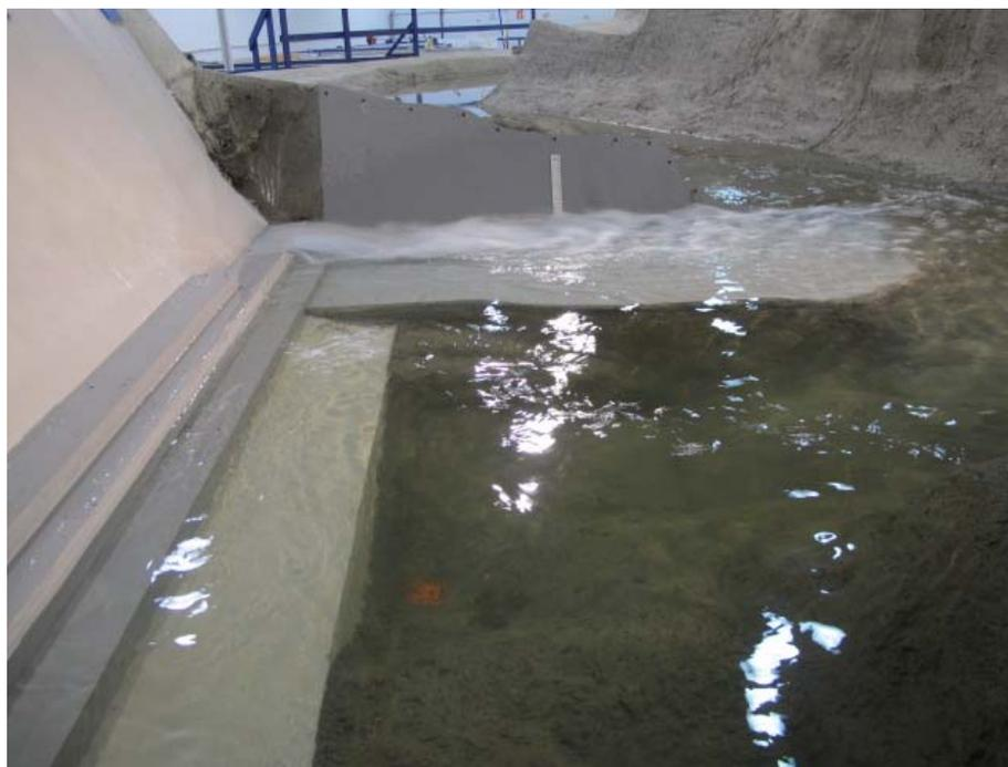
**Photo 2:** 1,000 cfs Spillway Discharge – Bay 8 – plunging flow.
