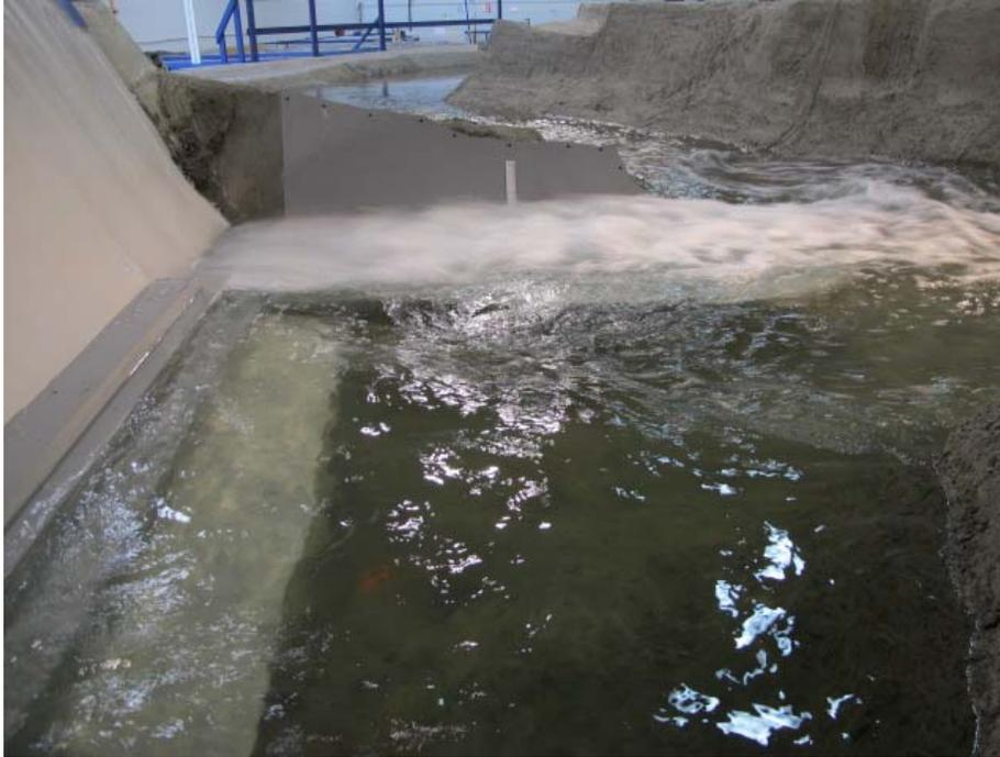
**Photo 3:** 5,000 cfs Spillway Discharge – Bays 7-8 – skimming flow regime.
