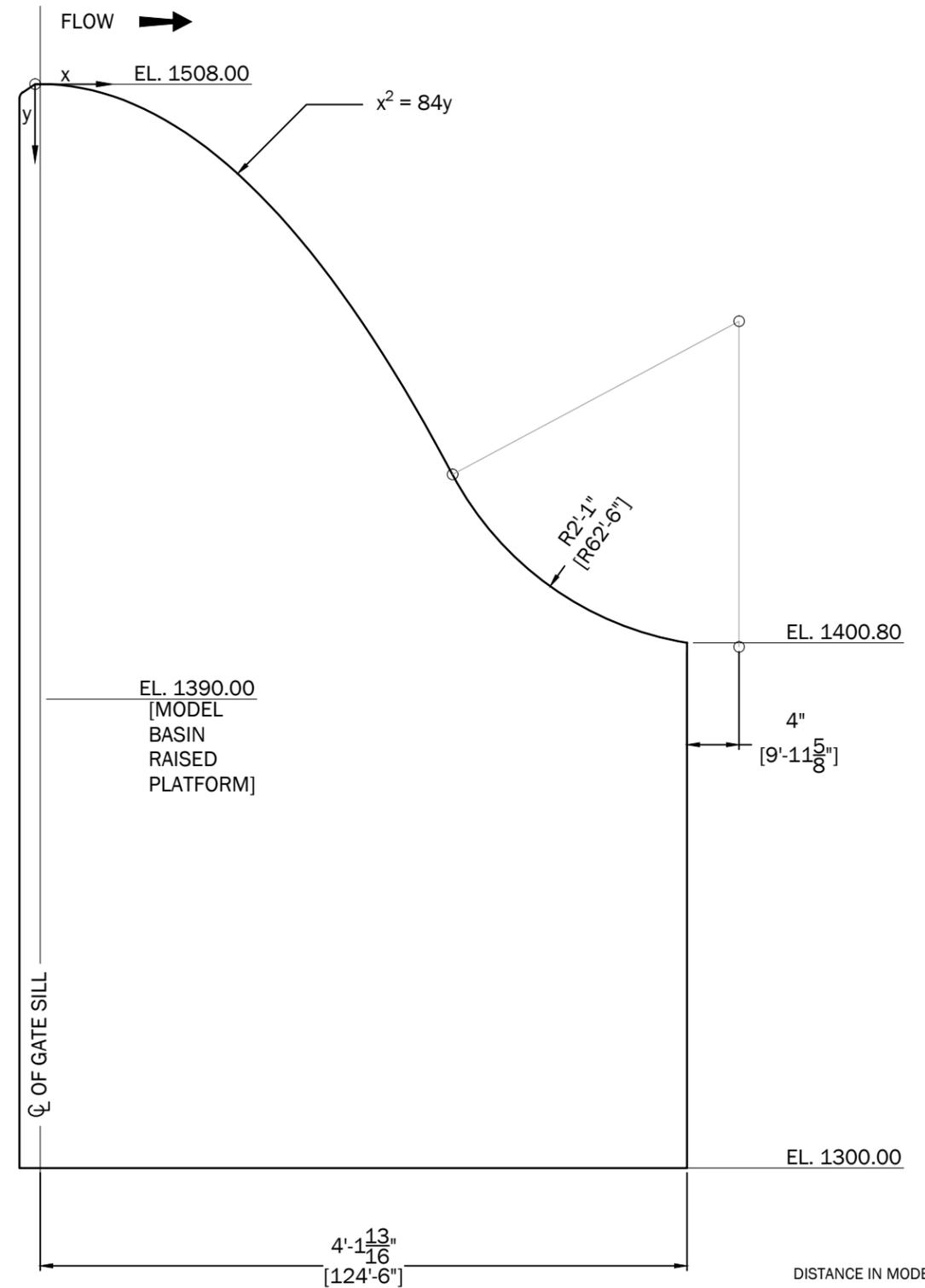
**3** TYPICAL SECTION - SPILLWAY: GATES 1 & 2
