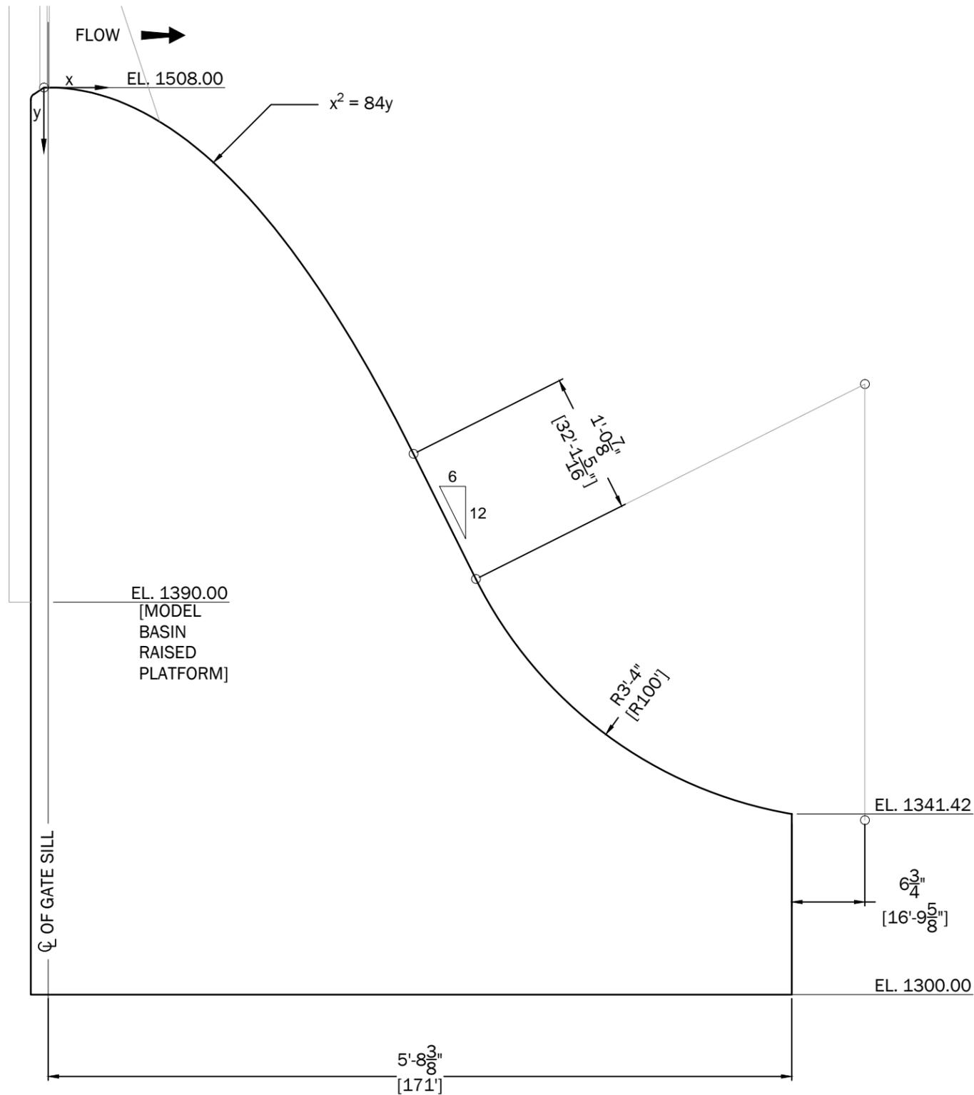
**2** TYPICAL SECTION - SPILLWAY: GATES 3, 4, 5, 6, 7 & 8
