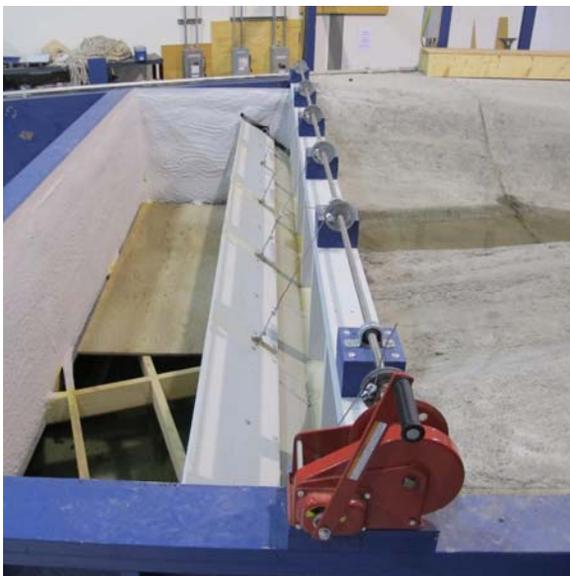
**Photo 7:** Tailgate which is used to control the tailwater condition.
