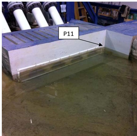
**Photo 8:** The model tailwater was measured at P11 near the powerhouse.
