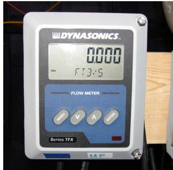
**Photo 4:** Dynasonic transit time flow meter for measuring flows.
