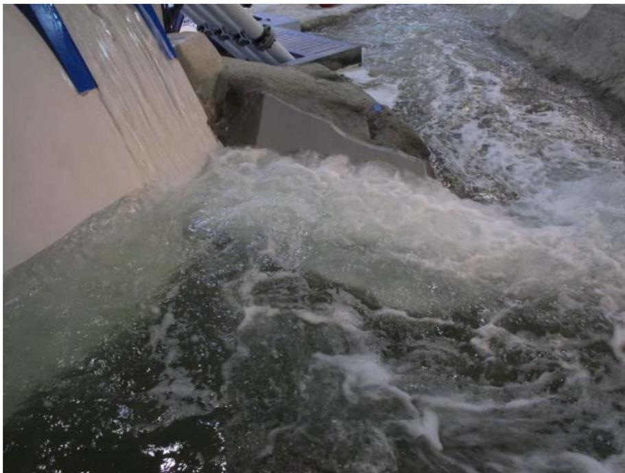
**Photo 2:** 25,000 cfs Spillway Discharge – Bays 7-8 – submerged surface jump flow regime
