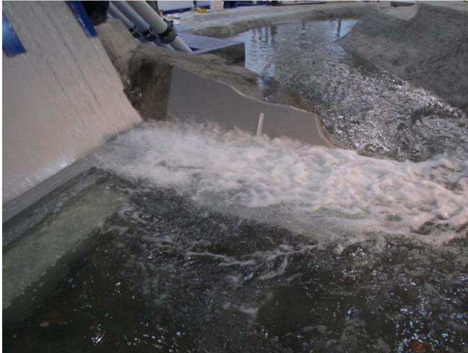
**Photo 1:** 5,000 cfs Spillway Discharge – Bays 7-8 – skimming flow regime.
