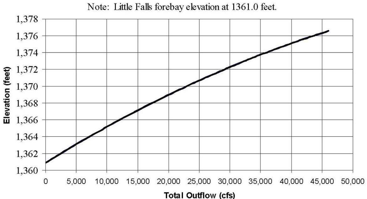
**Figure 1-2 Graph of Tailwater Surface Elevation below Long Lake Dam**
