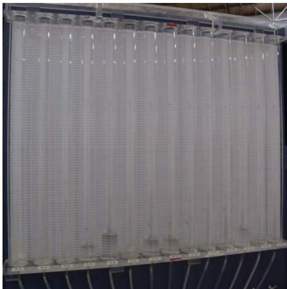
**Photo 3:** tilling wells used to measure pressure tap readings from the model.
