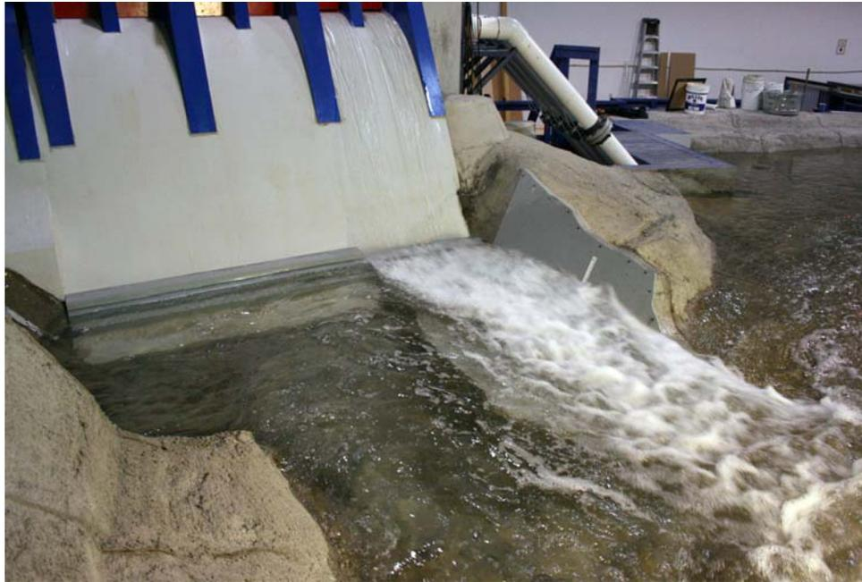
**Photo 1:** 5,000 cfs Spillway Discharge – Bays 7-8 – skimming flow
