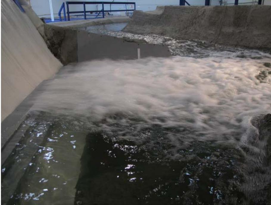
**Photo 5:** 10,000 cfs Spillway Discharge – Bays 5-8 – skimming (Bay 7&8), plunging (Bays 5&6)
