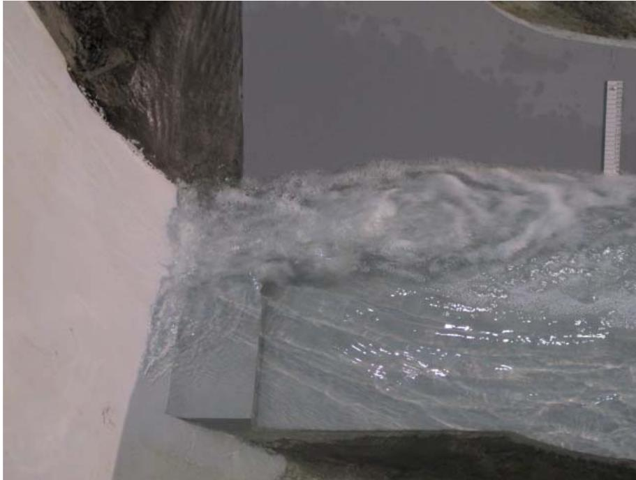
**Photo 1:** 1000 cfs Spillway Discharge – Bay 8 – submerged surface jump flow regime.
