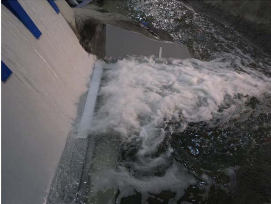
**Photo 1:** 10,000 cfs Spillway Discharge – Bays 5-8 – ramped surface jet flow regime.
