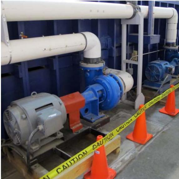
**Photo 1:** Two of the Three Laboratory pumps supplying water to the model.
