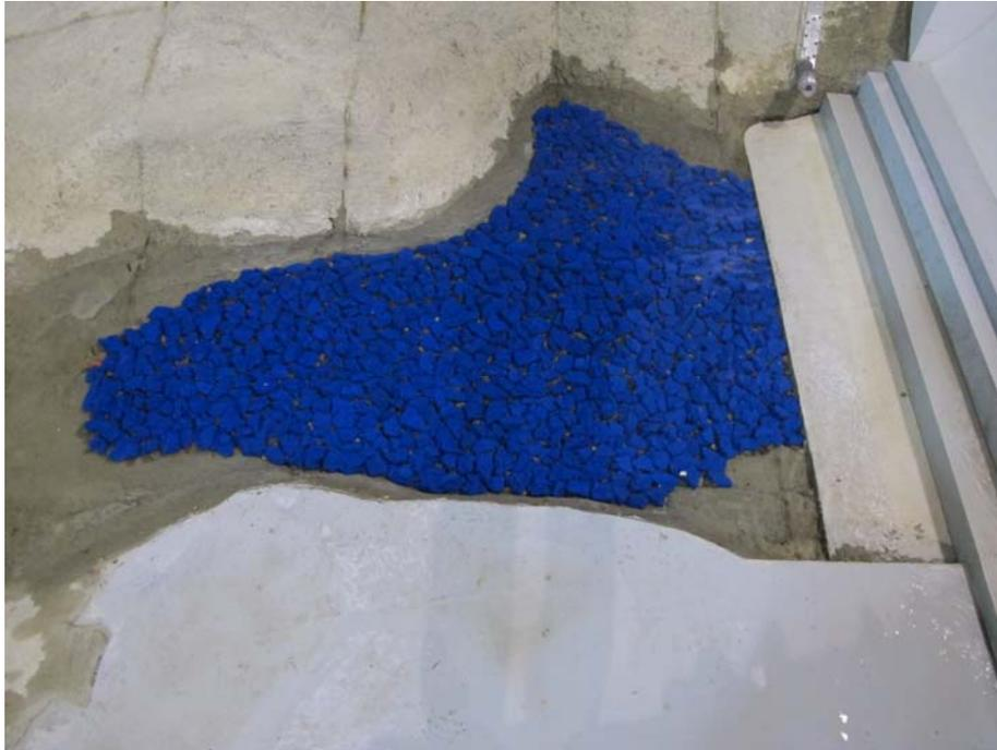
**Photo 1:** Mobile bed prior to 50,000 cfs discharge.
