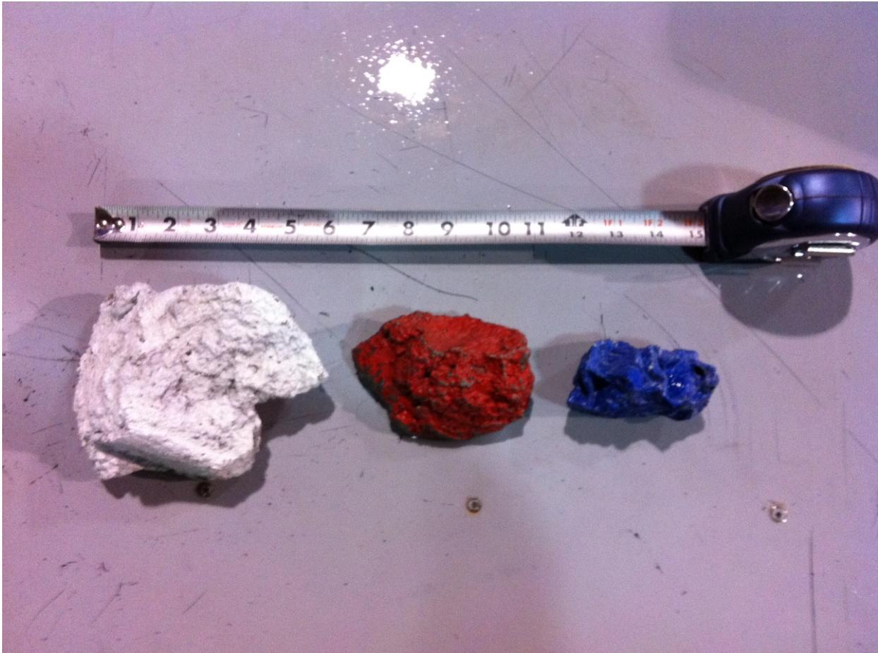
**Photo 1:** Different size classes of material used to test the stability of plunge pool fill material.
