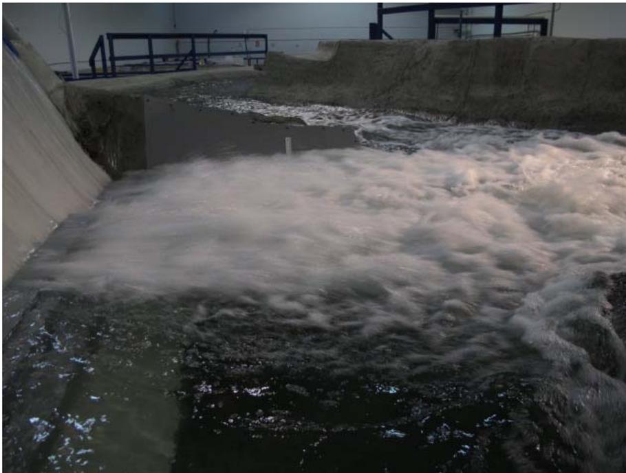
**Photo 6:** 16,000 cfs Spillway Discharge – Bays 5-8 – skimming to ramped surface jet.
