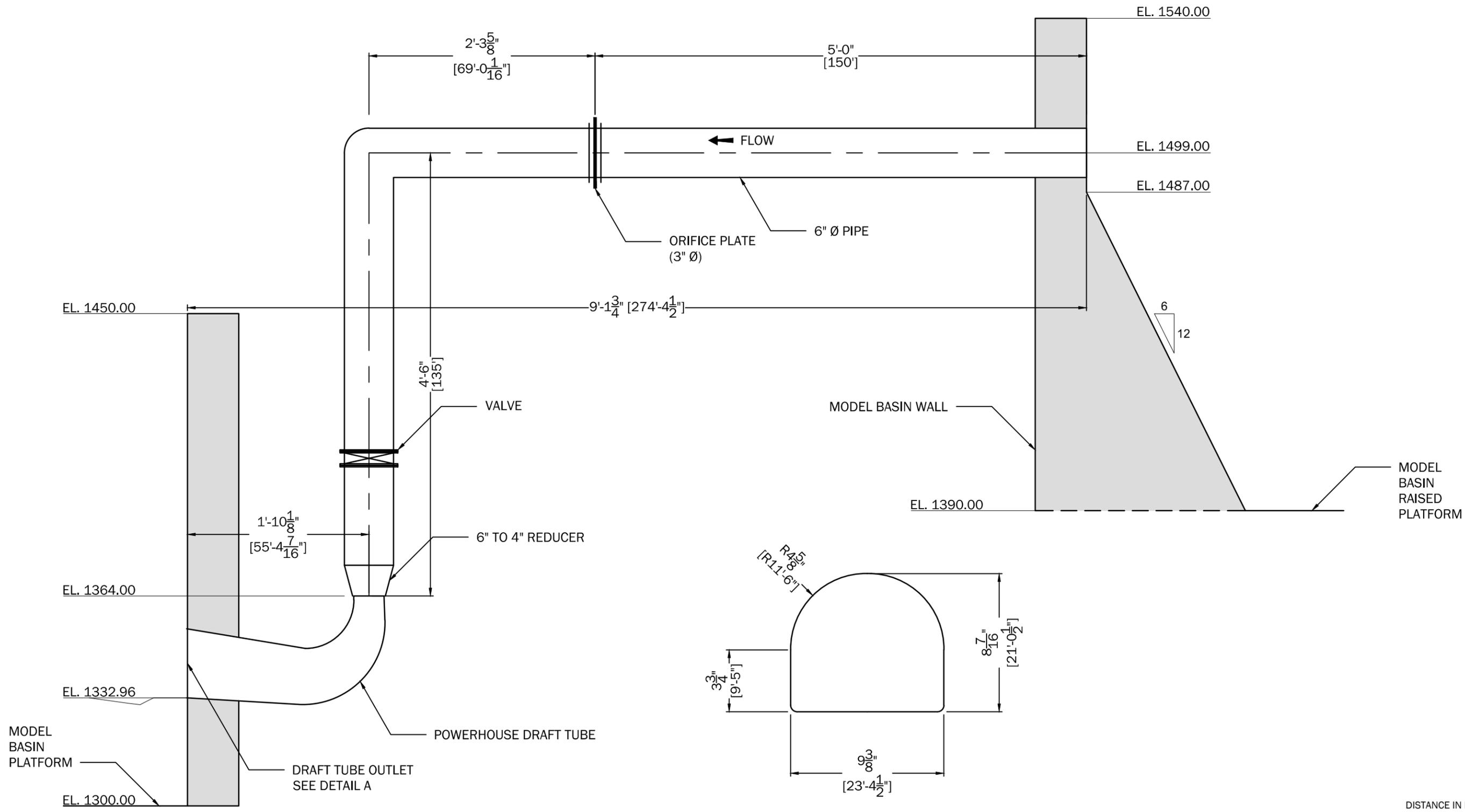
**1 TYPICAL SECTION - POWERHOUSE INLET AND DRAFT TUBE**
