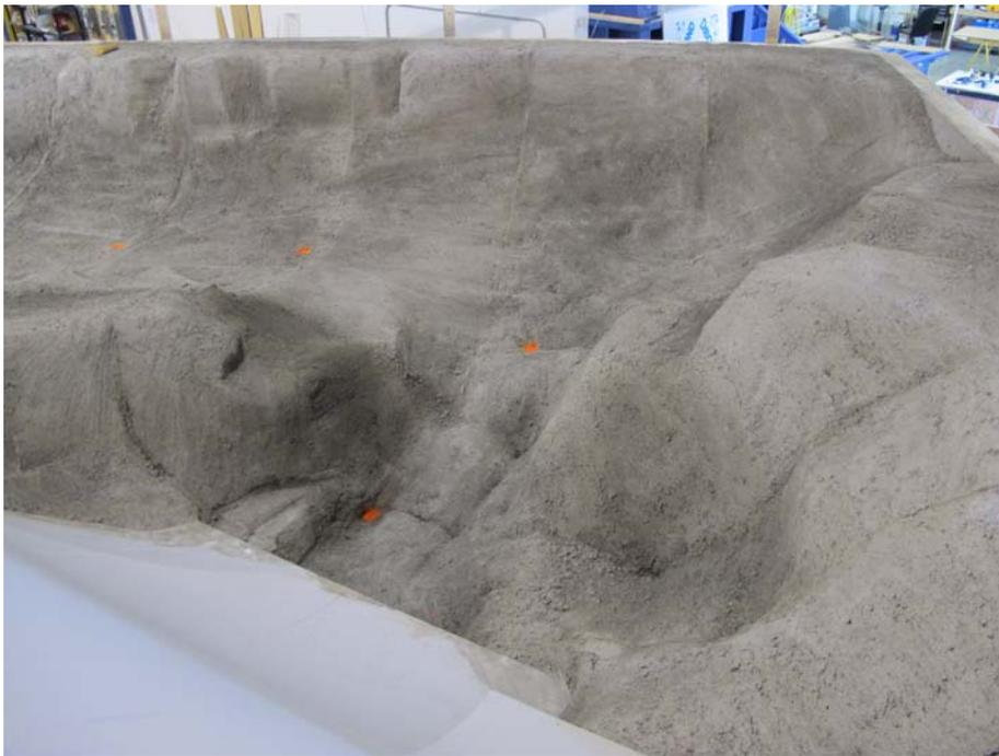
**Photo 2:** Downstream view of the plunge pool and spillway toe.
