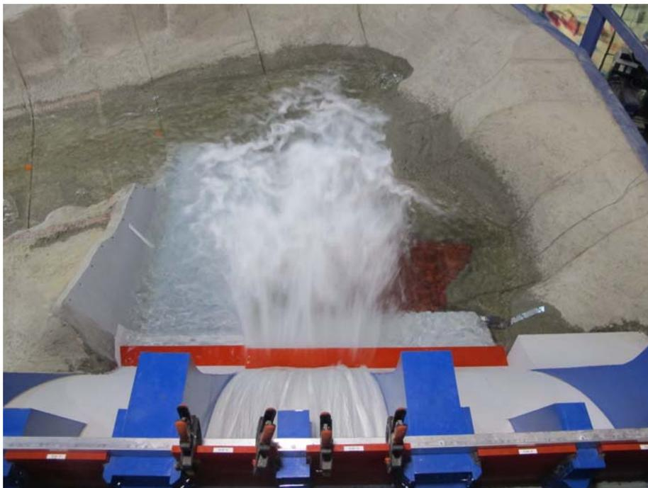
**Photo 2:** Looking downstream for the spillway crest at the plunge pool.
