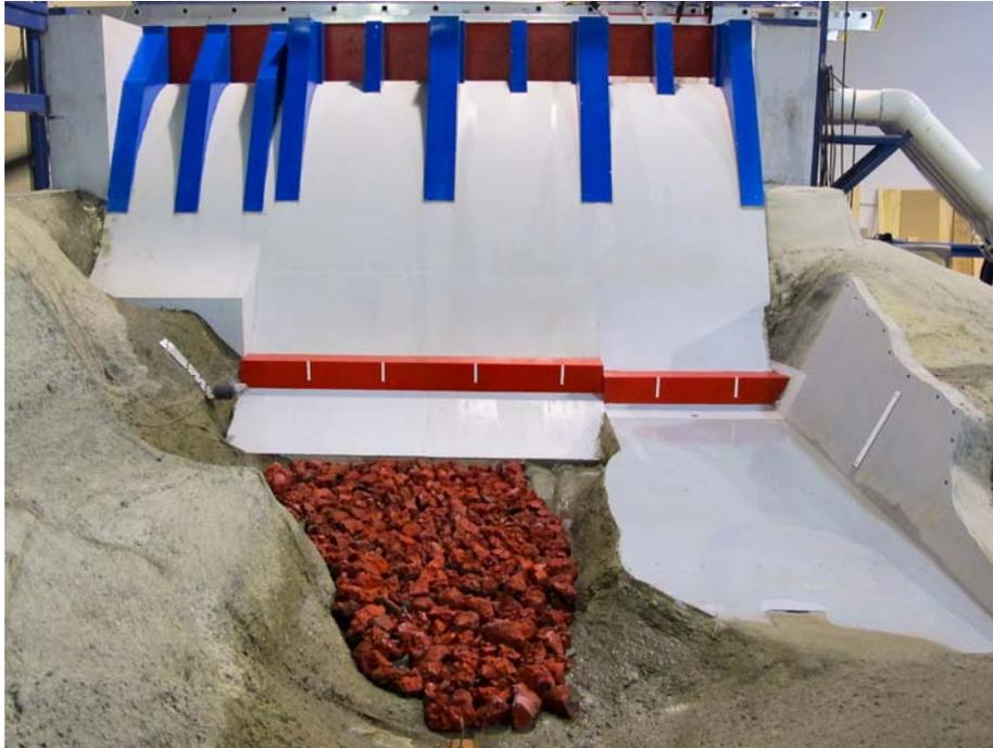
**Photo 1:** Alternative 1 spillway deflector final configuration with filled plunge pool.
