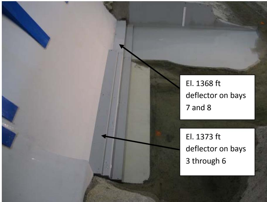
**Photo 1:** Elevation 1368 ft and 1373 ft deflectors, model not running.
