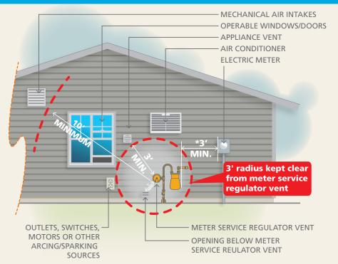
\*In Oregon, electric provider PP&L requires a 3-foot minimum horizontal distance to any part of the gas meter. In all other areas, a 3-foot radial distance from the meter service regulator vent is required.
