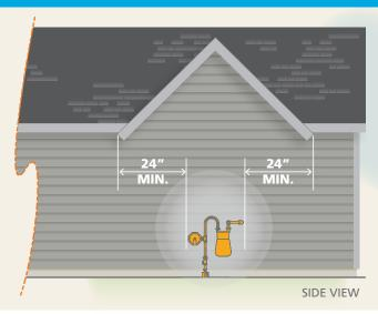
In areas prone to heavy snowfall (see below), protect the meter from snow and ice by locating it under a roof overhang of at least 12 inches from the dripline to the front face of the meter or on the gable end of the building. If this is not possible, a snow shed should be installed. Avista-provided snow sheds are the preferred option. The customer also may build and install their own Avista-approved snow shed (see design details at myavista.com/safety).
