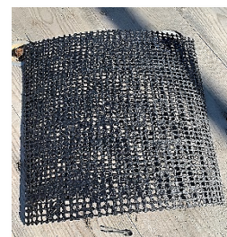
A piece of fire mesh wrap
