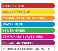
Ground markings are in different colors to indicate the locations and types of utility facilities buried below. Valid periods for locate marks are: WA - 45 days; ID - 21 days. If anyone digs after the listed times, they are digging with an invalid ticket.
